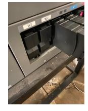
2. Remove the white ink cartridges from the printer.
