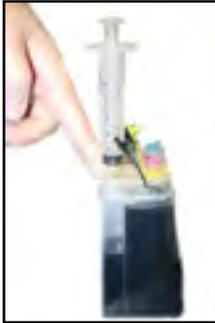
With the plunger already pushed into the syringe, attached the syringe thru the breather hole of the color you wish to prime (make sure you leave the filling hole plugged).
